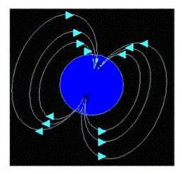
The earth's magnetism is caused by the flow of electrons in its fluid metallic core. The fluid core is perpectually in motion. This explains why the earth's magnetism varies with time. The move is quite gradual. Thus, the earth may be visualized as a huge magnet with its magnetic poles moving. The change in the location of the magnetic north is known to as **secular variation**.
